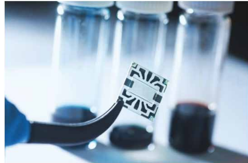
A new flexible graphene solar cell developed at MIT is seen in the transparent...
